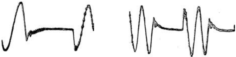
Left: Tone-burst test on medium-priced magnetic cartridge. Oscillogram shows marked 'ringing' up to high frequencies. Right: Ringing effect due to resonances in cheap magnetic.
