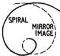
FIG. 63. THE DERIVATION OF CAM SHAPE.
