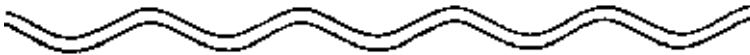
Fig 12 The same signal 'in phase' in each channel produces a groove that looks like this from above.
