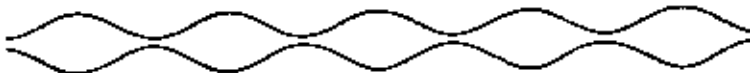
Fig 13 The same signal 'out-of-phase' in each channel produces a groove that looks like this from above.
