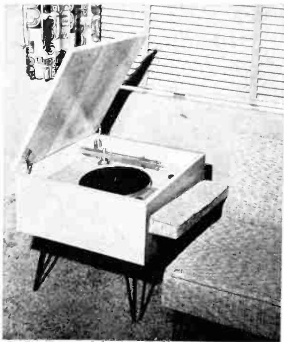
High quality single-play turntable is installed in shop-made cabinet on iron legs. WEINGARTEN ELECTRONICS, LOS ANGELES
