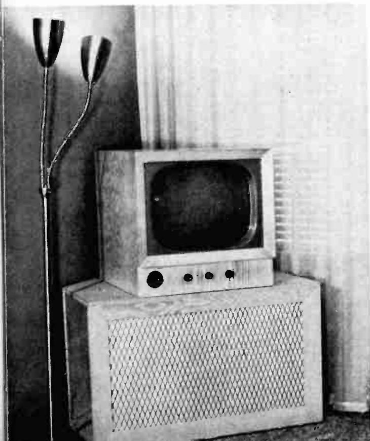
Custom built corner horn was designed to support table model TV set which is heard through the Hi Fi speaker enclosure. T & W Electronics, Inglewood, California.
