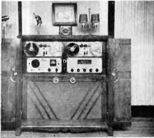
Dual tape recorders with tuner and preamplifier for continuous music. MAGNECORD, CHICAGO, ILL.
