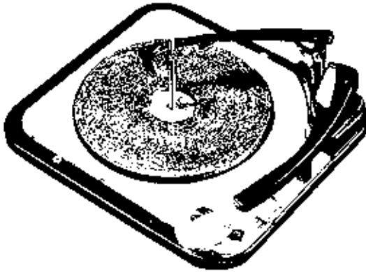
Fig. 4-13. A typical record changer.
