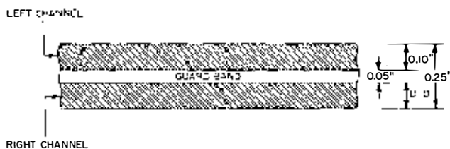
Fig. 3-11. Dimensions of tracks and guard band for two-track stereo tape.
