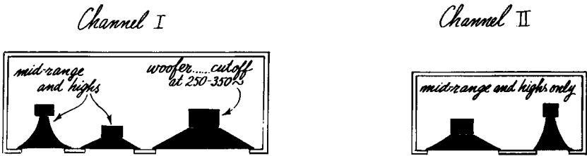
Fig. 121. Stereo setup using different speaker systems.
