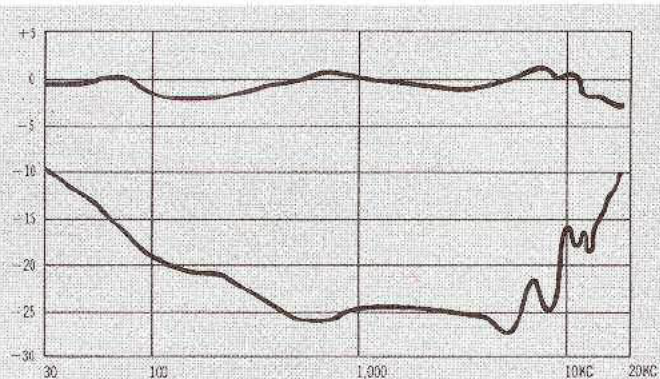
Typical frequency response and separation between channels of Model VR-227. (Performance of VR-225 exceeds the characteristics of the VR-227.)
