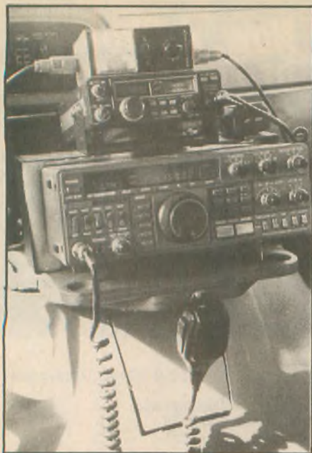
Top to bottom: SWR meter, Yaesu 230R and TS 430R stacked on a swivel plate on the mounting platform. There is a foam rubber cushion between the platform and the van engine cover.
