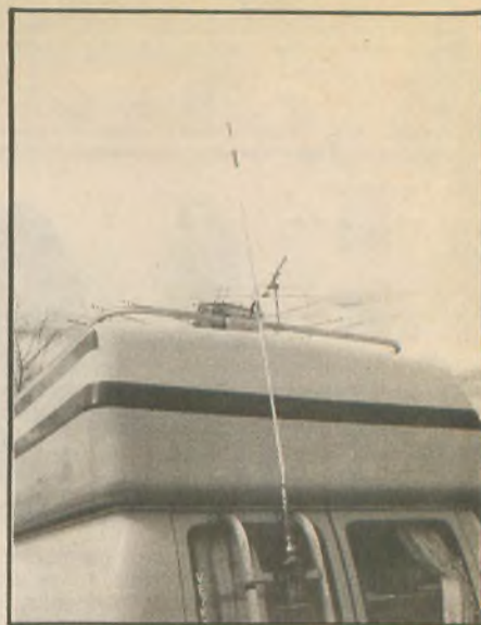
Optimal antenna location on the van: above resonator spring is 15M resonator with extended whip for 20M operation.
