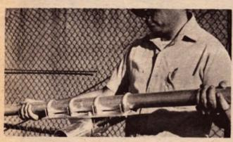
Our 40 meter element to boom clamps are constructed of aluminum bar plate 1/4" thick, 5" by 18" long. The element is secured with 6 ft. coupler and 4 full circle clamps to the mounting plate. Two 3" full circle clamps secure plate to boom.
