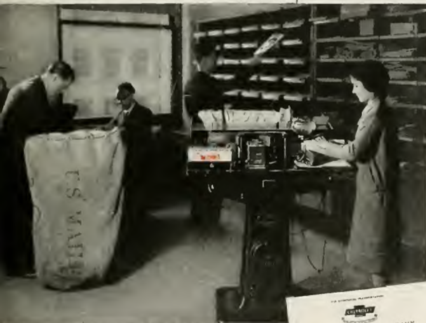
Chevrolet Motor Co. Mail Room, showing Pitney-Bowes Mailing Machine and Postage Meter in operation. This machine automatically feeds, separates, seals, postmarks, imprints postage and stacks mail - all in one operation.
