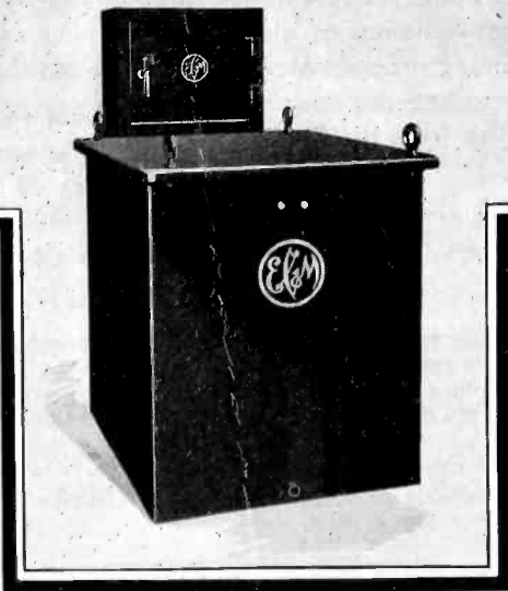
The single Type ZHS Magnetic Contactor, showing liberal electrical clearances, large bakelite barriers between phases and large contact areas.
