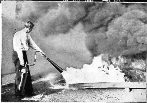
Attacking an oil fire with the B-1, C-1 LUX Standard Extinguisher. Note the white blanket of LUX gas.
