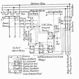
FIG. 11—DIRECTIONAL OVER-LOAD AND DIRECTIONAL GROUND PROTECTION
