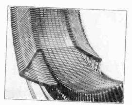
FIG. 11-PARTLY WOUND STATOR, SHOWING METHOD OF BRACING THE COILS
