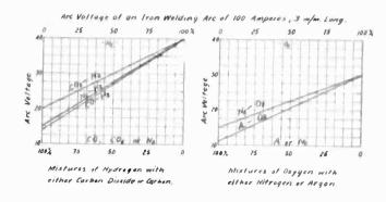
electrode and the arc core has the preponderent influence on the stability of the arc.
