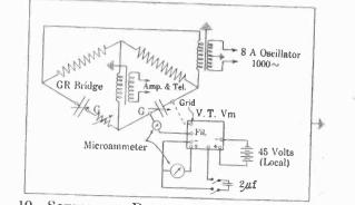
FIG. 10-SCHEMATIC DIAGRAM OF IMPEDANCE BRIDGE
