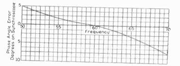
FIG. 12—SYNCHFOSCOPE CHARACTERISTIC One winding exciter from potential transformer One winding exciter from vacuum tube amplifier
