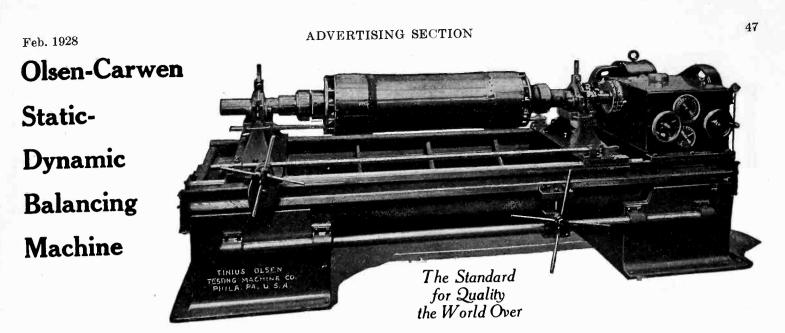
The OLSEN-CARWEN indicates unbalance both statically and dynamically in ounce inches on indicating dials, together with the angle or plane of unbalance; and also indicates the axial rotation of the static unbalance along the length of the rotor.
