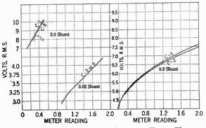
FIG. 7-SAMPLE CALIBRATION VACUUM TUBE VOLTMETER High range 1000 cycles High range zero = 0.14 on 0.02 shunt
