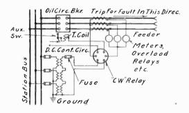
Fig. 14—Typical Diagram of Connections for the Residual Volt-Ampere Relay
