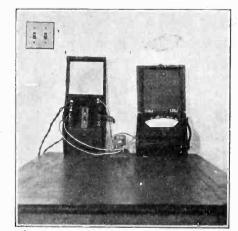
FIG. 4-CABINET, MICROAMMETER AND CONDENSER
