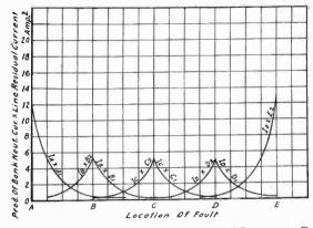
FIG. 13—PRODUCT OF TRANSFORMER BANK NEUTRAL CURRENTS AND RESIDUAL LINE CURRENTS
