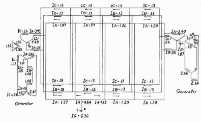
FIG. 7—FAULT-CURRENT DISTRIBUTION DIAGRAM
