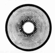
FIG. 1-HOLLOW CORE CABLE
