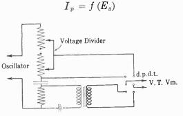
FIG. 12-CIRCUIT FOR MEASURING TRANSFORMER CHARACTERISTICS
