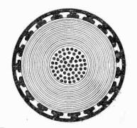
FIG. 2-SLOTTED SHEATH CABLE
