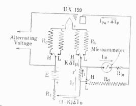
FIG. 1-SCHEMATIC DIAGRAM OF VACUUM TUBE VOLTMETER
