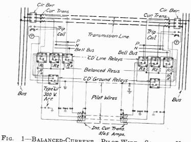
Fig. 1—Balanced-Current Pilot-Wire Scheme Using Selective Differential Relays
