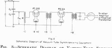
FIG. 8—SCHEMATIC DIAGRAM OF VACUUM-TUBE SYNCHROscope Equipment
