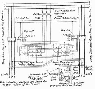
FIG. 2A-PROTECTION FOR A PAIR OF PARALLEL LINES
