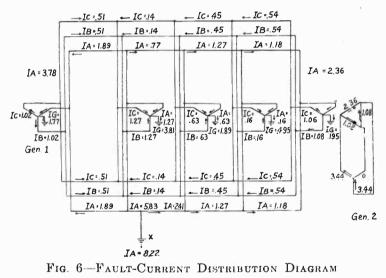
Showing effect of grounding the neutral of substation power banks
