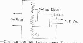
FIG. 11—COMPARISON OF IMPEDANCES USING VACUUM TUBE VOLTMETER
