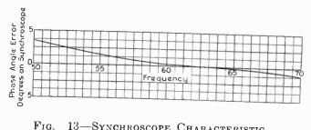
FIG. 13—SYNCHROSCOPE CHARACTERISTIC Excited from vacuum tube amplifier
