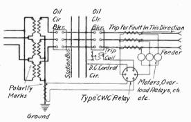
$F_{1G},\ 12-Typical Diagram$  of Connections for Ground Protection Using the Inverse Time, Residual, Over-Current, Ground Relay
