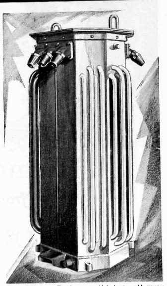
Wagner Subway-type Transformer assembled showing cable-entrance flanges and brass terminal bushings. Wiped joints are made between the lead sheaths of the cables and these bushings. Pressed copper terminals are sweated to the ends of the cable and bolted to studs on terminal board.
