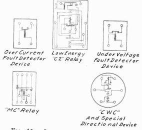
FIG. 15B-INTERNAL WIRING DIAGRAMS
