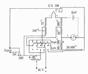
FIG. 3-WIRING DIAGRAM OF ASSEMBLED VOLTMETER
