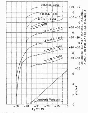
FIG. 13-VARIATION OF WAVE-FORM ERROR WITH BIAS
