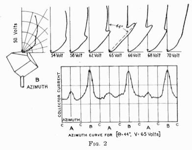
and Fig. 2, a typical set of experimental curves showing the gradual development of a spur of diffracted electrons at 50 deg. and 54 volts. The power curves show how this diffracted beam depends on the azimuth of the collector relative to the axes of the crystal structure.
