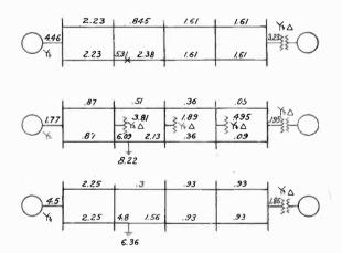
FIG. 8—A COMPARISON OF FAULT-CURRENT DISTRIBUTION WITH IDENTICAL FAULT LOCATION
