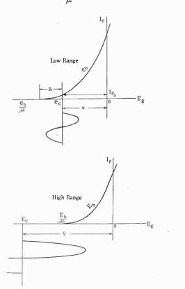
FIG. 2—THE DOUBLE-RANGE DESIGN  $e_b$  = plate battery voltage = plate filament voltage  $e_c$  = operating bias  $\mu$  = voltage amplification factor of tube
