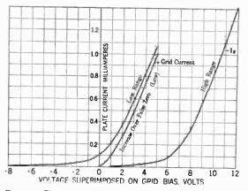
FIG. 14-STATIC CHARACTERISTICS OF VACUUM TUBE VOLTMETER
