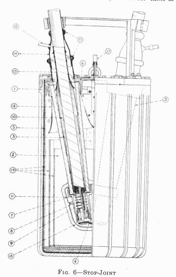
suitable thickness and has a lining, 5, hermetically sealed to the upper cover, 6. The terminal's insulators are cemented at the upper end to the cover and are provided at the lower part with two cemented metal caps, 7; the tightness of the seams is guaranteed by composition cork gaskets.
