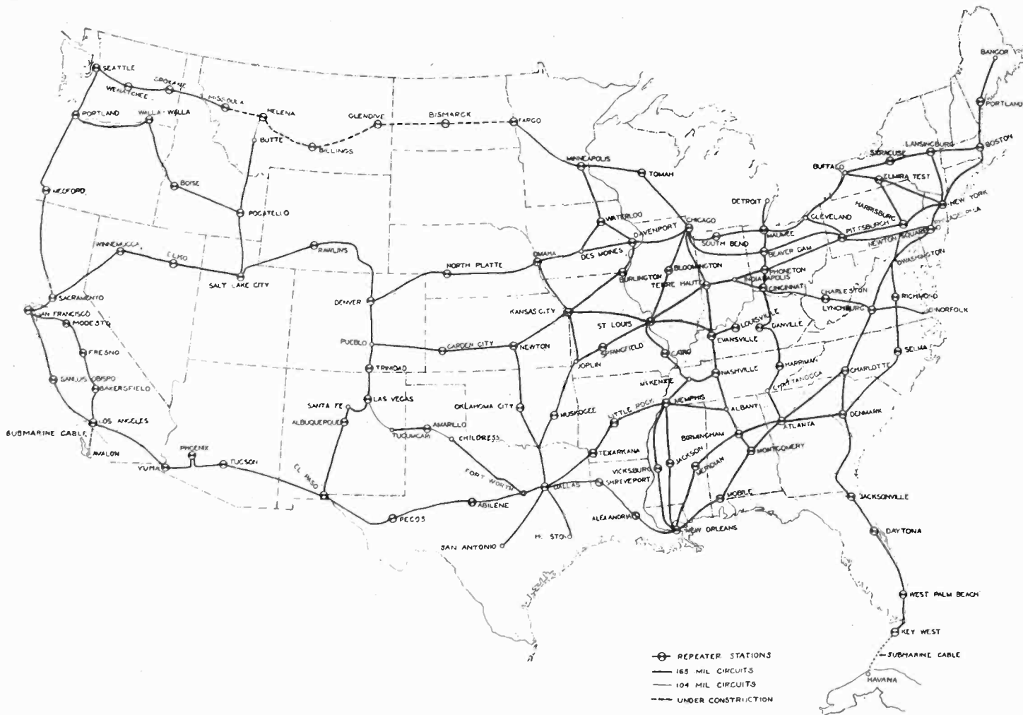
FIG. 1—ROUTES OF TRANSCONTINENTAL-TYPE TELEPHONE CIRCUITS IN THE UNITED STATES
