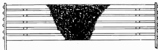
FIG. 20—DUMMY CONNECTIONS SHOWING BURNED PORTION
