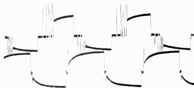
FIG. 6—OSCILLOGRAM SHOWING CURRENT FROM ARMATURE CONTACTS
