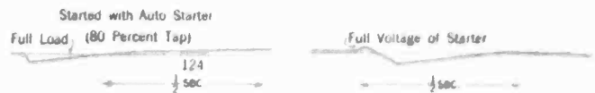
FIG. 4A—COIL MOVEMENT OF 50-H. P., 440-VOLT, 60-CYCLE MOTOR WHEN STARTED WITH STANDARD AUTO-TRANSFORMER
