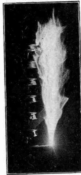
FIG. 10—DRY 60-CYCLE SPARK-OVER OF A SHIELDED STRING OF INSULATORS Arc clears the string
