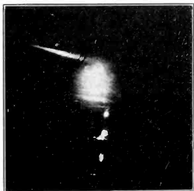
FIG. 36—PHOTOGRAPH OF ARC OVER THREE SUSPENSION INSULATOR DISKS. REACTOR SETTING 811 OHMS
