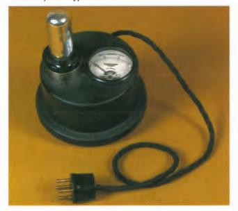
Test unit for 199 type tube.
