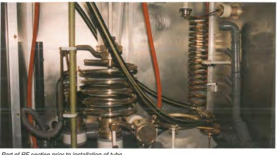
Part of RF section prior to installation of tube.
