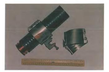
Wind-induced vibration has caused fatigue failure of stainless steel cable clamp.
