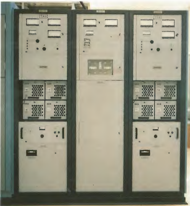
New Nautel 2x5 kW transmitter.
