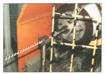
Application of helix to centre conductor of FLEXWELL HF 7/8 inch Cu2Y cable.
