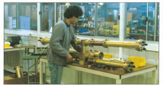
Assembly and testing of 16 way UHF power divider for China.
