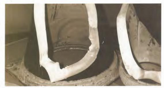
Damaged armature support insulator 4QG/4QR Bald Hills due to lightning stroke.
