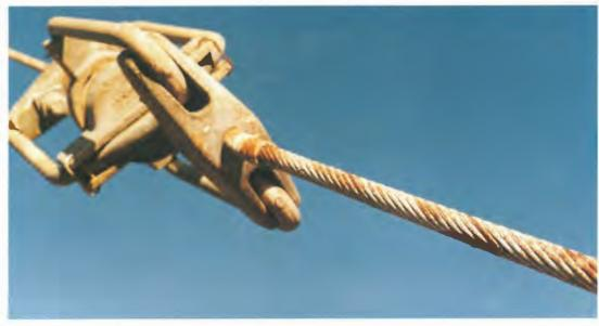
Guy rope and insulator assembly corrosion 7NT Kelso.
