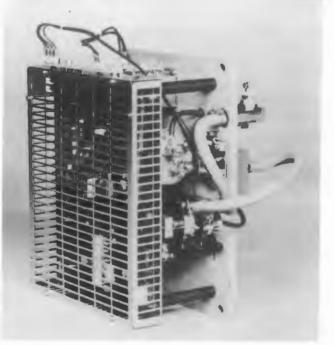
Partial front view PSM amplifier showing pulse frequency filter and some switching stages. (Courtesy Brown Boveri & Co.)
