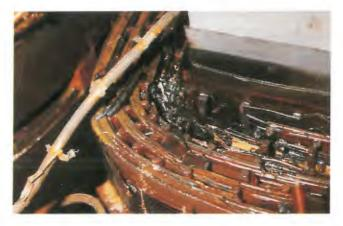
Damage to secondary winding.
