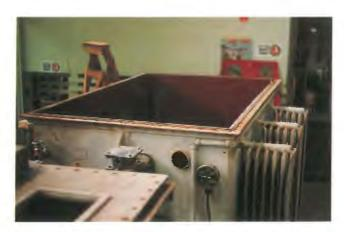
Transformer tank with core removed.
