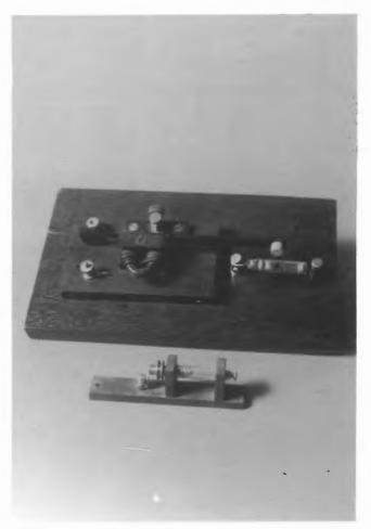
Two coherers. Hammer type (top) and rotating type.
