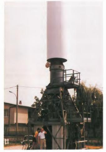
Antenna rotator with UHF antenna mounted for test.
