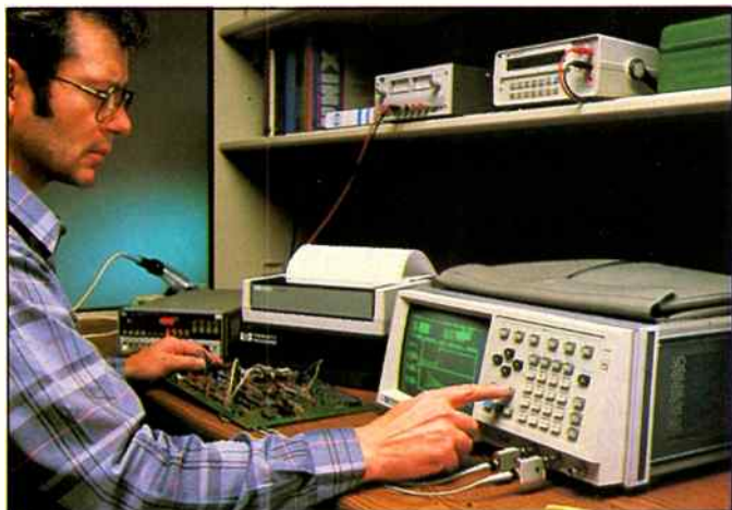
Sophisticated! Heart of the system here is a high performance programmable digitising oscilloscope with VDU-type screen, teamed with a printer and other programmable instruments forming part of a system. (Hewlett Packard photograph.)
