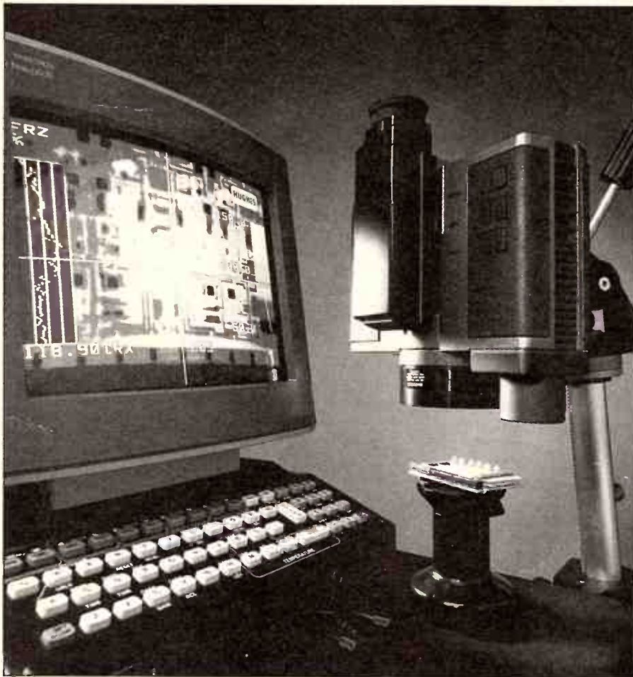
You can get a "macro" view, too. Here, the Hughes thermal video imaging system is looking inside a hybrid circuit in operation.
