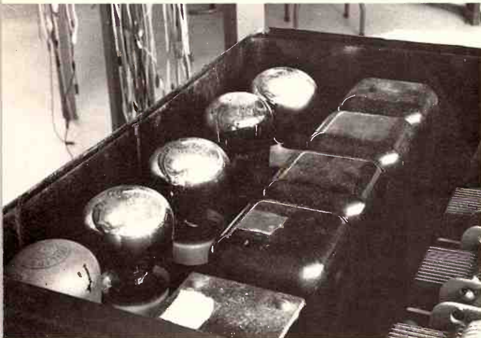
Part of Stromberg Carlson's 7-valve radio. RF section on the left, tuned coils in centre, 4 gang tuning capacitor on the right. Mains-operated, valves are 4 pin or 5 pin.
