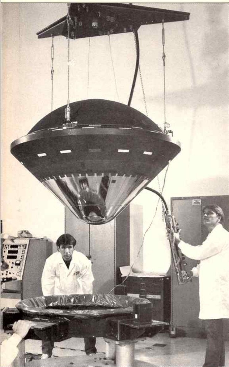
Technicians at Hughes Aircraft Company's Los Angeles plant complete final tests on the Galileo Probe which is scheduled to enter the atmosphere of Jupiter in late 1995. Weighing around 330 kg now, the probe will experience deceleration forces so great on encounter with Jupiter's atmosphere that its weight will increase to the equivalent of a DC-10 aircraft. Carrying scientific instruments, it will parachute through the fiery atmosphere for about an hour, transmitting valuable data to the Galileo Orbiter spacecraft which will carry it into space in October.
