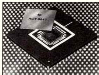
The single-chip, floating point processor
