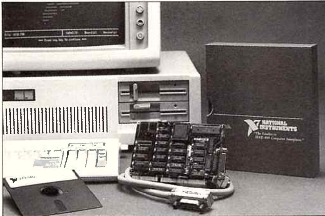
The AT-GPIB from National Instruments — a high-speed IEEE-488 interface.
