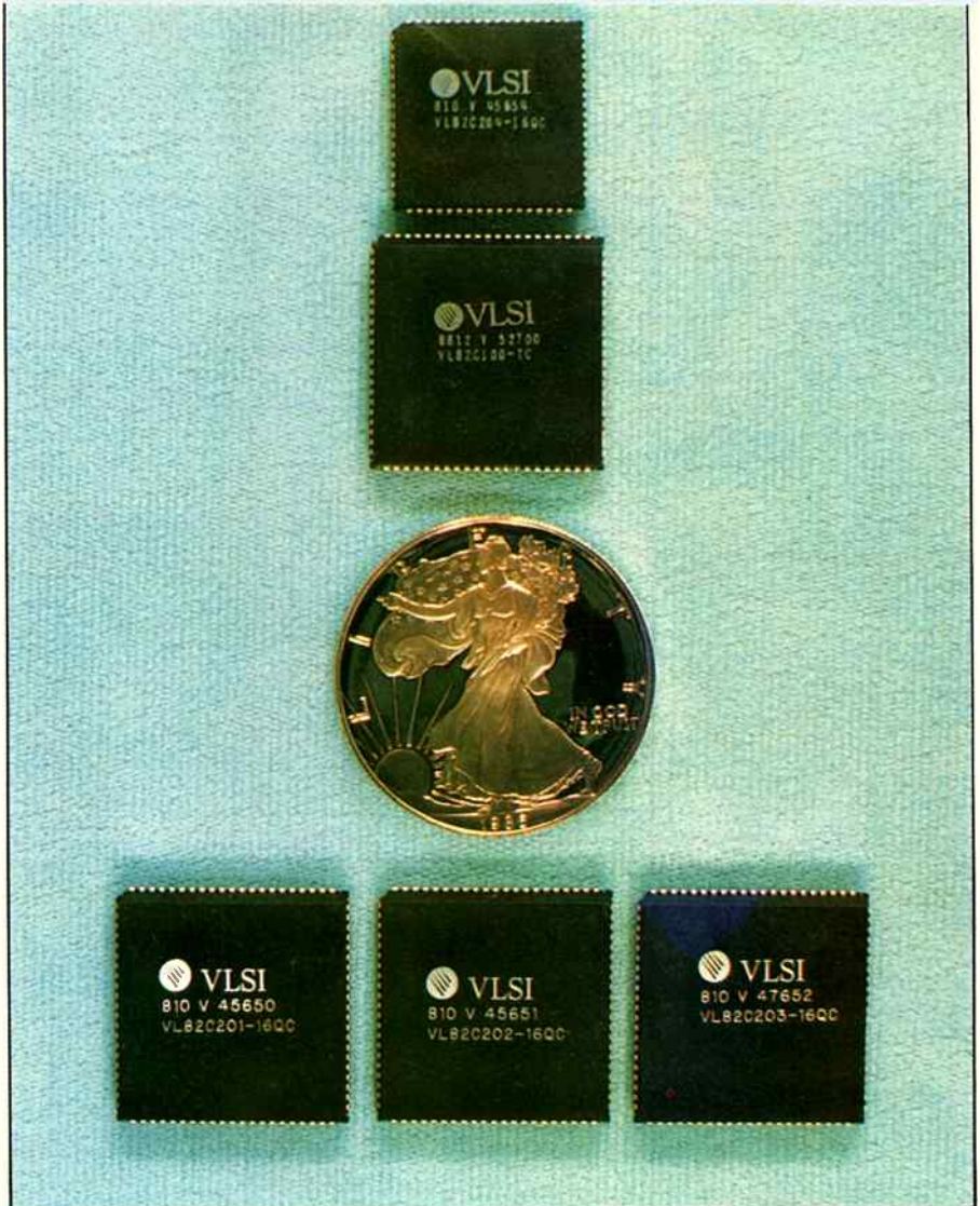
Five chips contain the majority of the circuitry to implement an entire AT.
