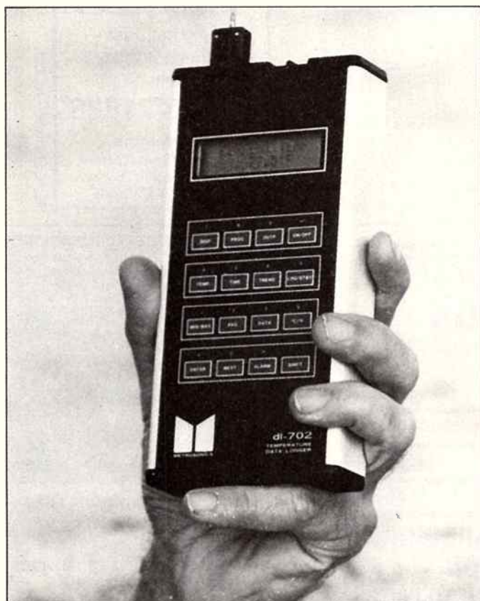
Point of measurement temperature logger by Metrosonics.
