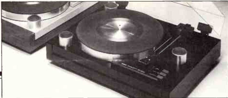
Two turntables from the Japanese Yamaha Music that use a two piece design for the platter. The two materials are chosen so that the resonance frequencies are different. The PF 800 (right) uses zinc and aluminium, while the PF 1000 uses gun metal and aluminium. In a rather cunning innovation, the belt drive is coupled to the inner of the two pieces, so that the effective inertia of the platter is increased without increasing its mass. This reduces flutter considerably. READER INFO No. 32
