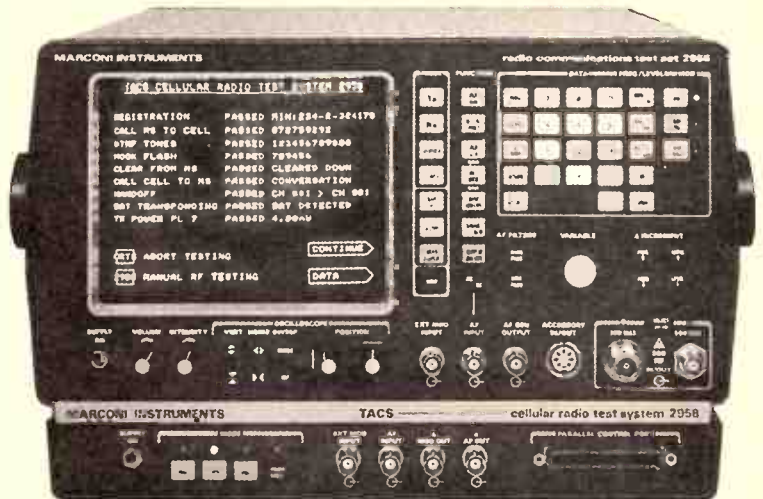
A cellular radio test set. An adaptor, the Marconi 2958 talks to the Marconi 2955 via GPIB
