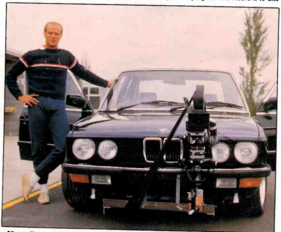
35 mm film camera rigged to the front of the BMW 635 for shooting at Sandown. Film was transferred to video disc for use in driving simulator.
