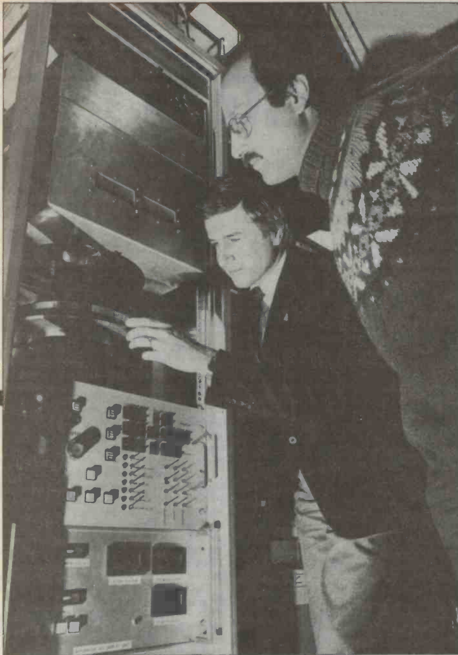
Chris Horwitz and Stefan Boronkay of Labtam with the hollow cathode etcher. Boronkay is touching the lower of the two cathodes. In operation, it slides up towards the compartment above, which is a vacuum chamber. Below is timing and other control equipment.
