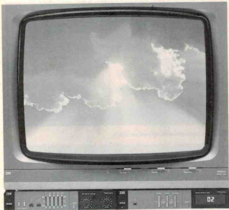
Audio Video Integration: video tuner on the right, preamp on the left.
