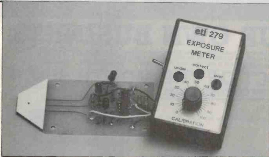
Insides out. The switch mounts on the side of the box and the battery slips in cross-wise. The pc board becomes the bottom, replacing the box's original lid.
