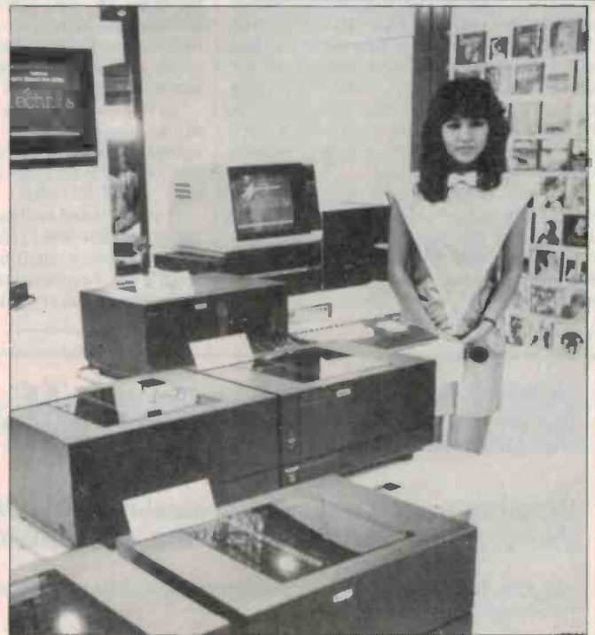
The Technics multiplay system consisting of a player that can take 51 compact discs, and four add-on modules that take 50 each!
