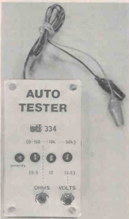
Pragmatic. Simple, but functional. The project was housed in a small jiffy box with a Scotchcal panel added.
