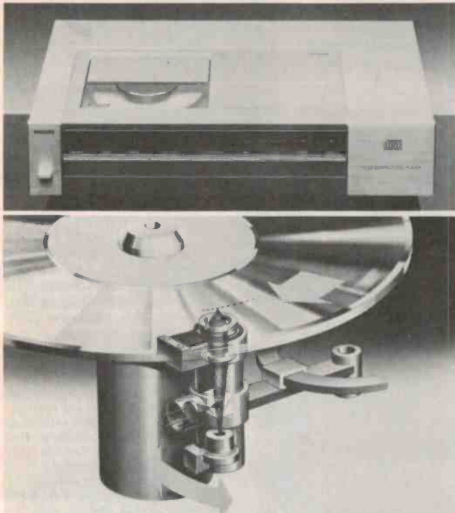
The disc is 'read' by focussing the laser light through the underside of the disc and optically reading the reflections.
