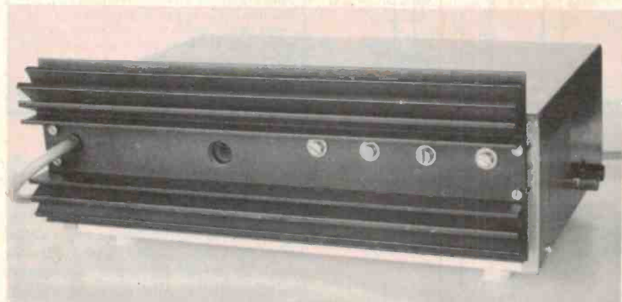
Rear view of the amplifier. Note the access hole for the Lo-Z output socket in the heatsink, just left of centre, and the line output terminals protruding from the right hand side of the case.
