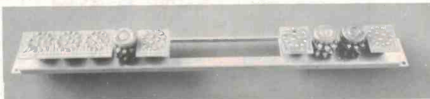
Rear view of the sub-panel assembly, prior to wiring.
