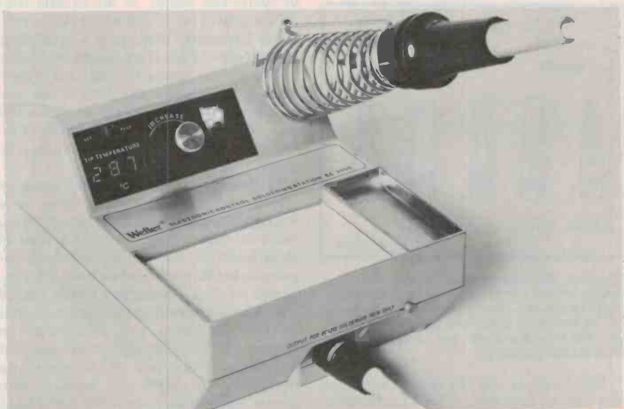
Figure 7. This iron, Weller's model EC2000D, employs a temperature sensor in the tip and electronic control of the power to the heating element to maintain the tip temperature within very close limits. The desired temperature is set by a knob and displayed in the three-digit readout.
