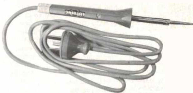
Figure 3. A popular continuous heat general purpose soldering iron, from Lotring. It has a heating element in the barrel and a tapered solid copper bit fits inside this, secured by a small grub screw at the end of the barrel. You can make your own bits for this sort of iron from copper rod.
