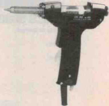
Figure 39. This Hakko 'Vac Ace' desoldering tool from G.E.S. employs a small vacuum pump to draw molten solder from the joint into the glass barrel atop the gun handle. A steel wool wad absorbs the solder. This tool is particularly effective on through-hole plated pc boards.
