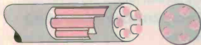
Figure 2. Construction of a 5-core multicore solder. The flux cores are located near the surface so that they melt faster, giving rapid fluxing action.
