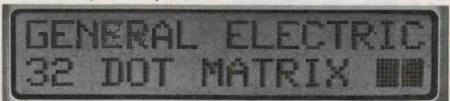
This 32-character liquid crystal display can produce numbers and letters on a 5 x 7 dot matrix in any of the 32 individual character cells. The device is made by General Electric and is model 95E from their GE-LXD product line.
