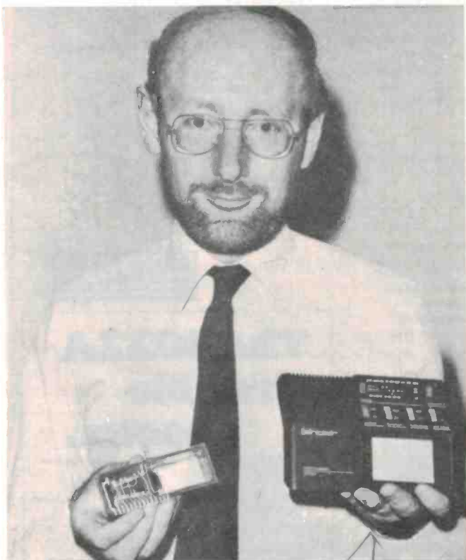
Clive Sinclair has finally produced his long-time 'dream', a tiny, portable, go-anywhere-in-the-world TV receiver. It is built around his flat screen cathode ray tube — which has much wider application if development continues.
