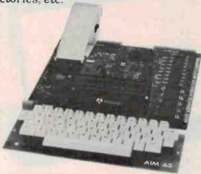
The Rockwell AIM 65 low-cost microcomputer, which incorporates a bubble memory.
