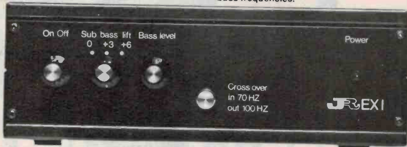
JR's electronic crossover unit for use with the Super Woofer
