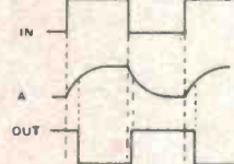
Figure 8. How to obtain a delayed and inverted version of an input pulse.
