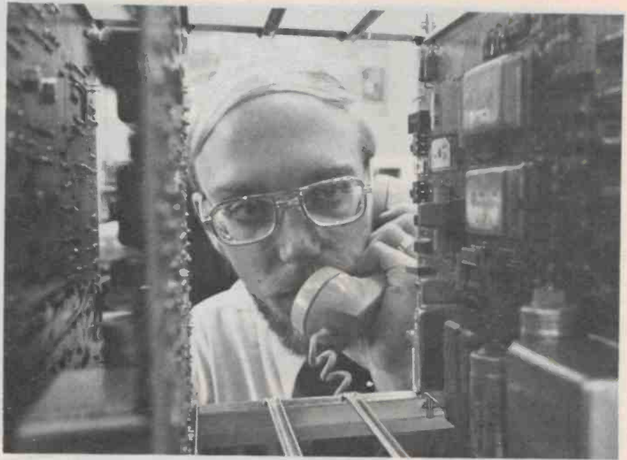
A Bell Laboratories engineer recording a 24-second message in the two magnetic bubble memories on the centre of the right-hand circuit panel.
