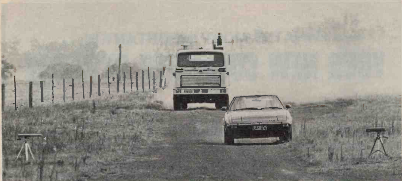
This photograph shows an actual measurement under controlled conditions of a situation similar to that described in Figure 2, below. The Mazda RX-7 in the front was driving at 25 kph while the truck behind it was travelling in excess of 65 kph. At the time this picture was taken the truck was several hundred metres behind the Mazda. The radar unit we used (electronics similar to the KR-11) clocked the truck's speed exclusively. The tripod at right carries a laser, the tripod at left a photodetector. A vehicle breaking the beam triggers a measurement on the set-up shown below.
