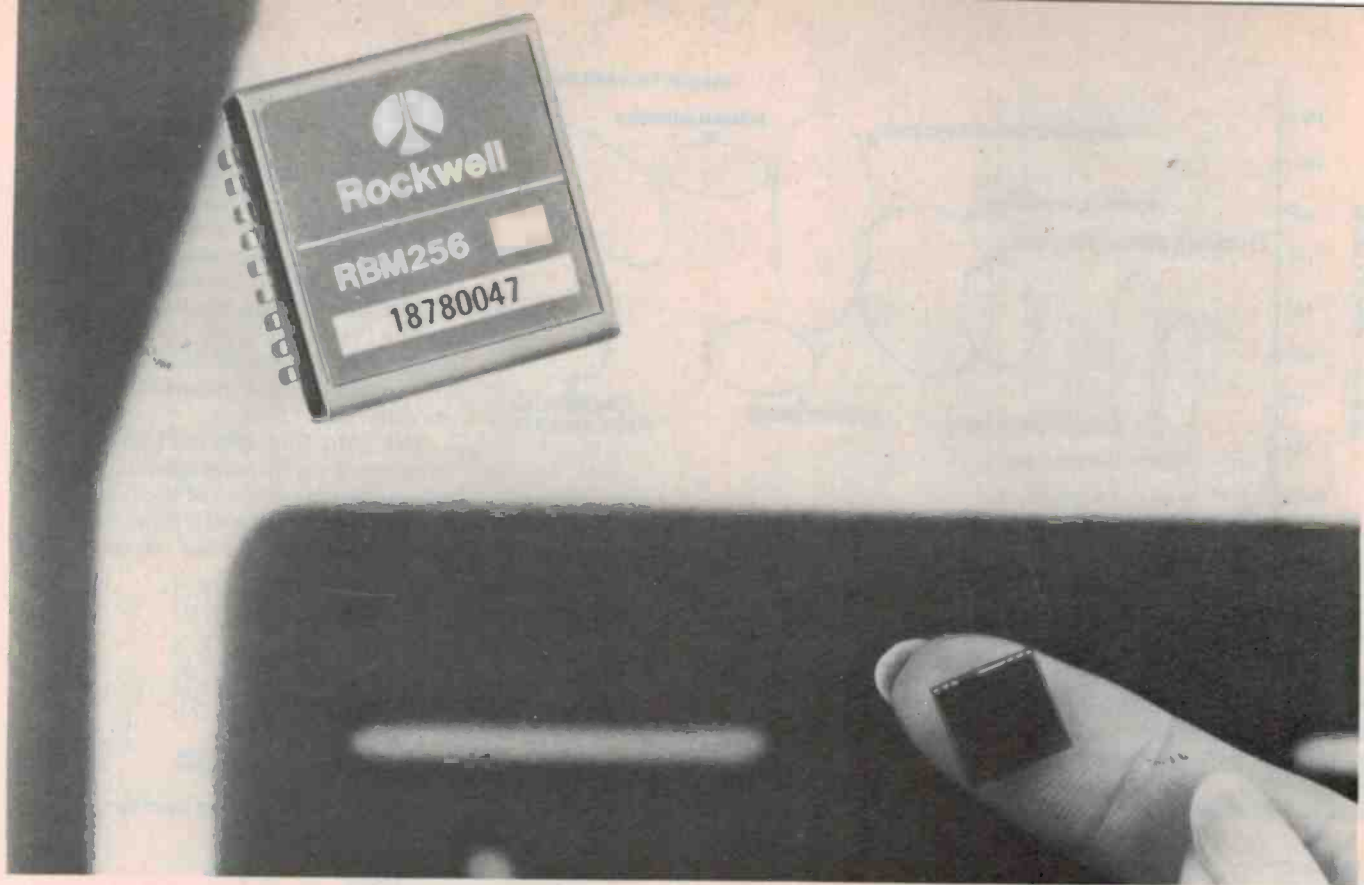
Rockwell 256 kilobit bubble memory type RBM256, photographed with a bubble memory chip on a finger, against a background showing a magnified part of the bubble chip's circuitry.
