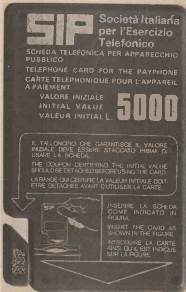
The 'electronic credit card' produced by SGS-ATES of Milan. They will be used with pre-paid telephones. It contains a 136-bit non-volatile memory arranged in a 17 x 8 bit configuration.
