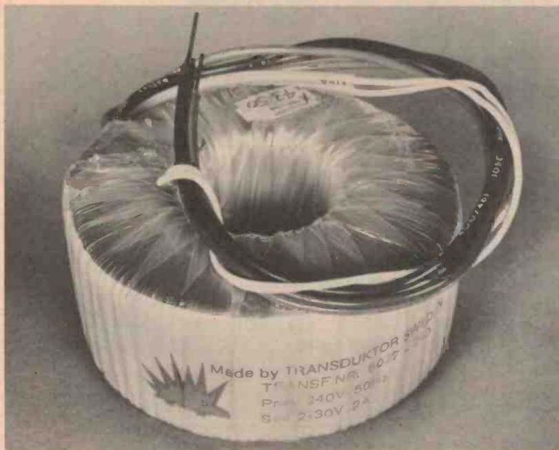
To get the maximum in hum suppression in your homebrew hi-fi amp, a toroidal transformer is recommended. This one suits the Series 4000 amp (with slight mods to the power supply). It delivers 30 V + 30 V @ 2A (240 Vac pri.) and costs $43.50 from Electronic Agencies, 115-117 Parramatta Rd, Concord NSW, 2137.
