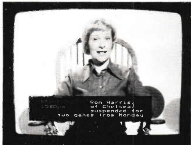
A major attraction of Teletext is likely to be the Newsflash. Receivers will probably be designed to enable the viewer to choose for Newsflashes to be superimposed on a regular programme either in a box as shown or in white.
