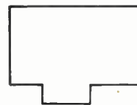
Fig 3 Details of heat sink shown full size, two required material tinfoil or thin copper.
