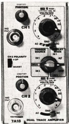
Fig. 11. Example of dual-trace plug-in showing the basic controls.
