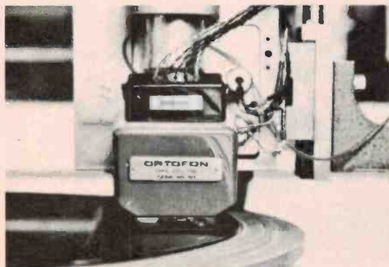
Ortofon professional cutter head type DSS 732 in action.
