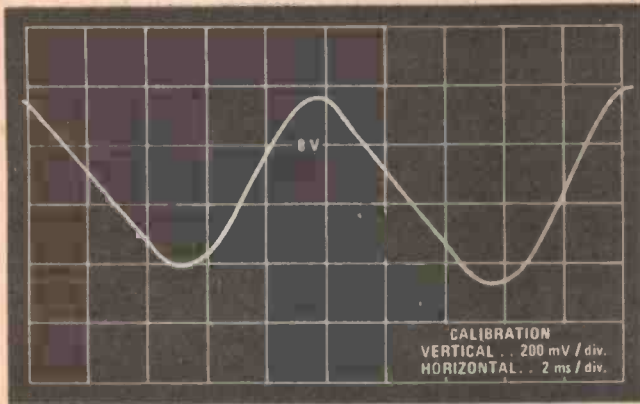
Fig. 2a. Ripple voltage on 8 volt output at 7.5 amps.
