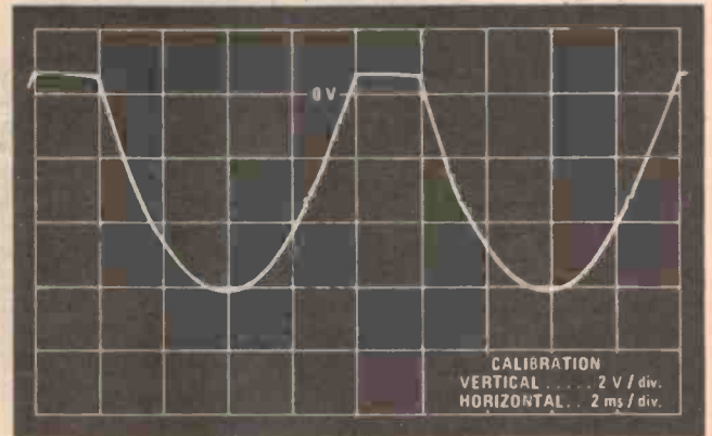
Fig. 2d. Waveform on the base of Q3.
