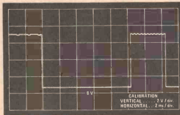
Fig. 2c. Waveform on pin 3 of IC1. On these waveform diagrams the beat rate has been increased to show the two different outputs available.
