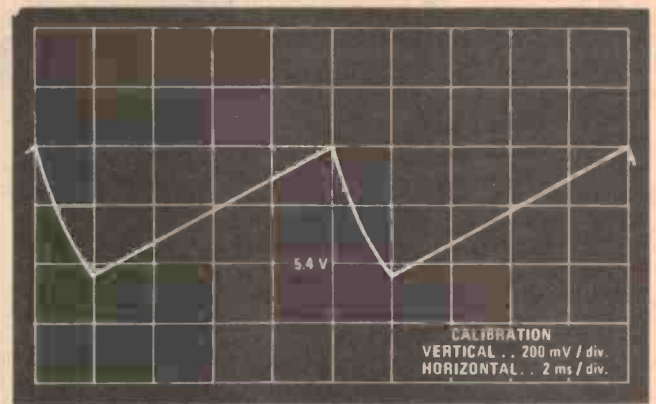
Fig. 2c. Waveform on the base of Q2.
