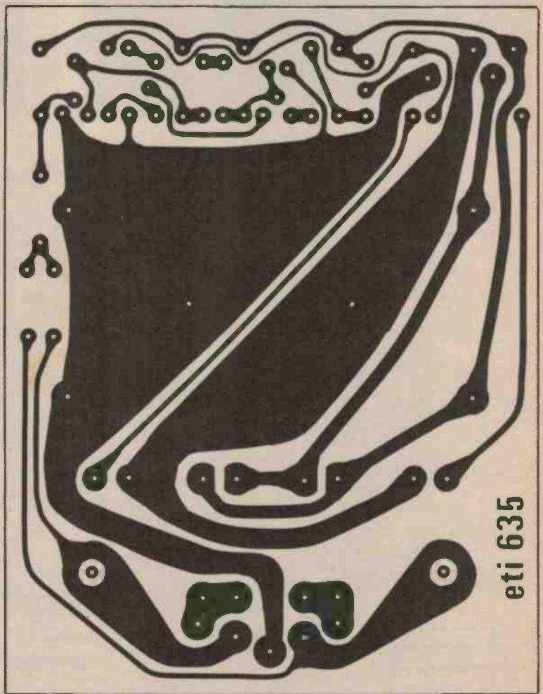
Fig. 1. Printed circuit layout. Full size 130 x 100 mm.
