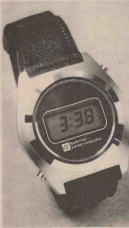
A typical LCD (Liquid Crystal Display) used in watches because of its low power consumption and ability to be seen in all light conditions.
