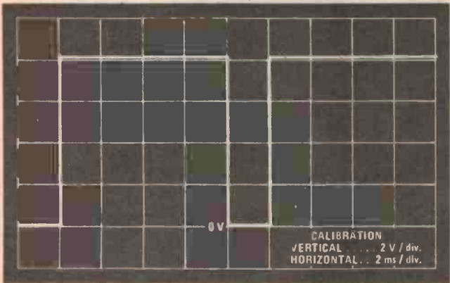
Fig. 2b. Sync pulse output.
