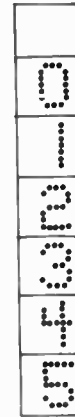
Fig. 14. A large size (38 mm character) alpha-numeric display constructed from discrete LEDs and a decoder/driver IC. (HP5082-7500).
