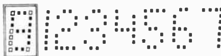
Fig. 6. Typical format of characters of the hexadecimal system using a 4 by 7 dot matrix.
