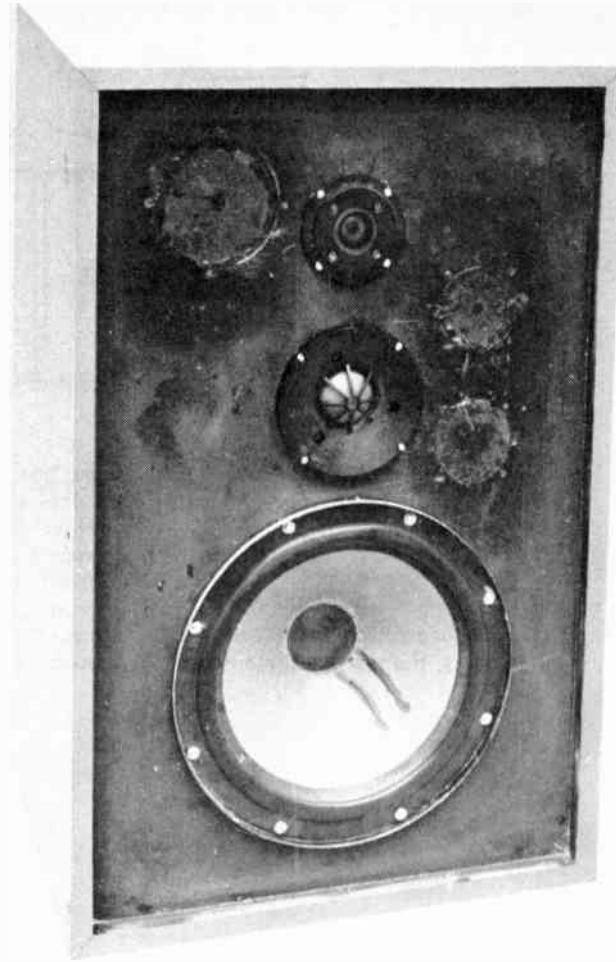
The prototype speaker with grille removed. The plugged holes were for trial positioning of midrange and tweeter.
