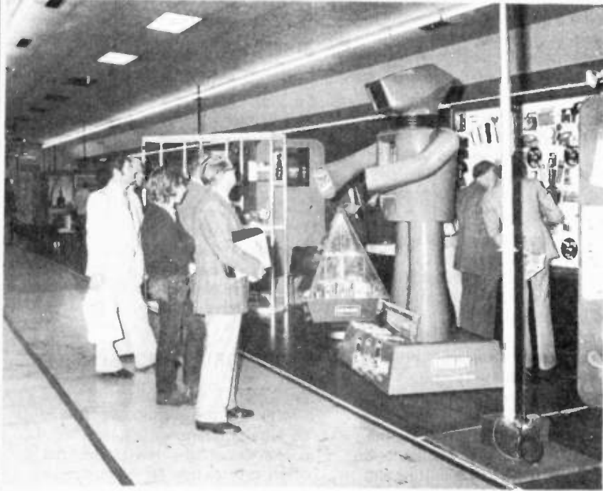
Star of the recent IREE symposium and exhibition was Union Carbide's robot ALFRED. The two and a half metre tall robot had a digital and alphabetical readout at the end of each arm to display answers to questions asked by visitors. A closed circuit colour TV camera in ALFRED's head enabled him to look at people to whom he was talking.
