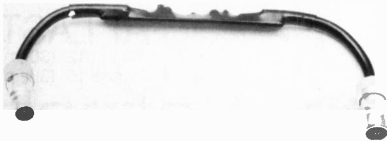
A simple low band attenuator which reduces channels by 24 dB.
