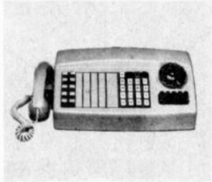
'PABX'—manufactured by Plessey Telecommunication Systems, this private automatic branch exchange system employs crossbar switching and componentry similar to that used by the Australian Post Office in the national telephone network.
