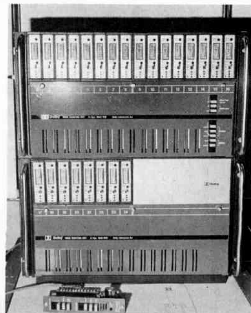
Fig. 6b. Bank of 24 Dolby A noise reduction units for use with 24-track tape machine.
