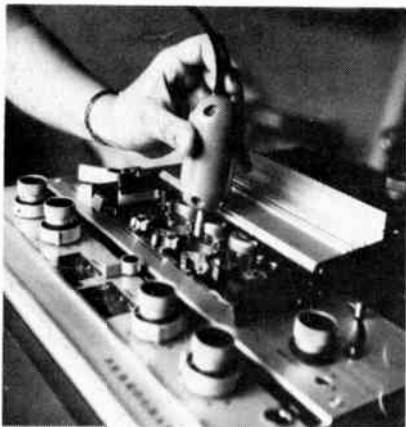
Fig. 1 Using a Defluxer to degauss the record head of a Ferrograph tape recorder.
