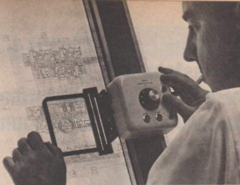
Layout of CMOS process masks is considerably enhanced by this coordinate digitizer machine. It is a convenient, efficient method for converting the designer's signal routing plan into data that a computer can understand and follow.
