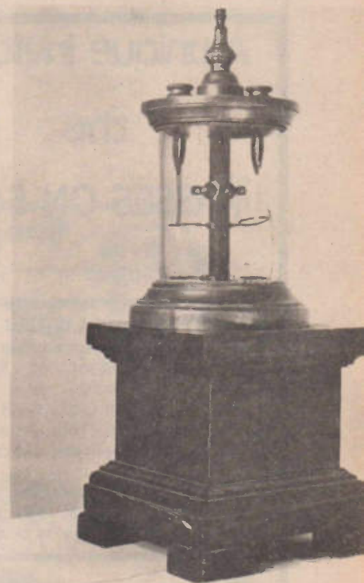
Fig. 4. This elegant coal-gas monitor of the 1900's has two treated papers hanging in front of the gas stream. The sampled gas passes through to be burnt at the top.
