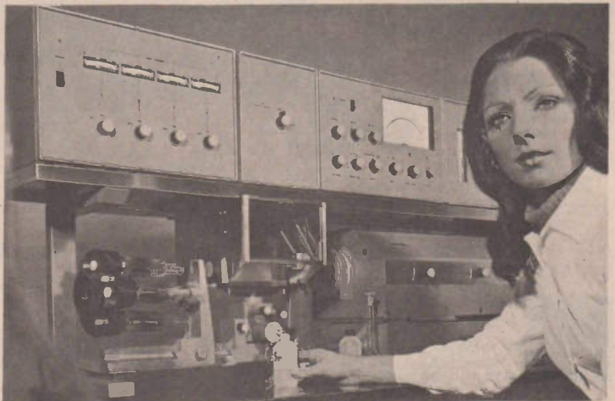
Fig. 8. The Australian designed atomic-absorption flame spectrophotometer.
