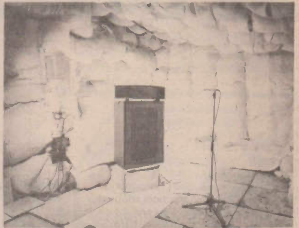
A speaker is born! This is the prototype for the Model 70 Electrostatic undergoing tests in John Bower's Anechoic Chamber.
